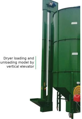
Dryer loading and unloading model by means of a belt elevator
