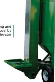
Dryer loading and unloading model by means of a belt elevator
