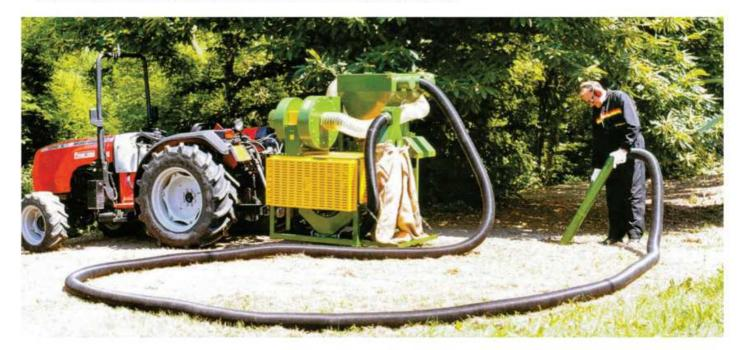
The machine can be used either for the picking of hazelnuts, using the anti-dust aspirator and the selection roller with 26 mm holes diameter. or for the picking of chestnuts using a selection roller with 45 mm holes diameter.
