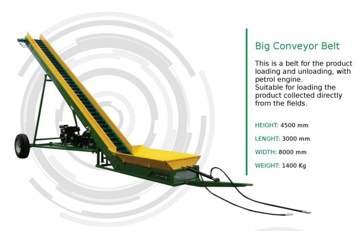
This conveyor is transportable with agricultural tractors directly in the fields to speed up the load of the product on the means of transport.
