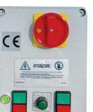
Control panel with potentiometer for electronic variator
